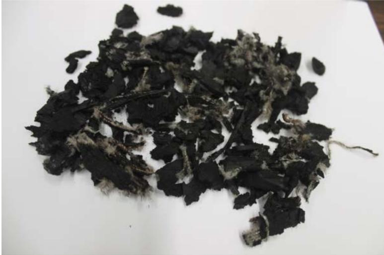
**Figure 3: Recycled Rubber Pieces Graded #6 (3.36 mm)**
