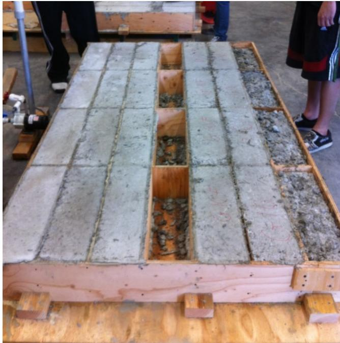
Batches were designed with an abbreviation to easily identify and differentiate each batch. The first letter of the designation describes the aggregate content, a C represents the control (unmodified aggregate), and a G for aggregate replacement with rubber. The second designation being the amount of rubber, either 10, 15% (by volume). Finally, if fibers were used in the mix, an F was added to the end of the designation.
