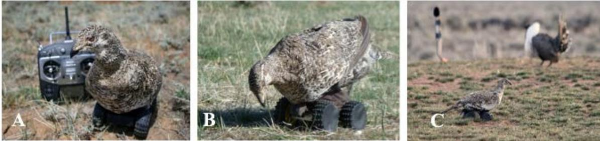
The leftmost panel (A) shows the robot in an up-right posture (or “interested” position) with the remote controller in the background; the middle panel (B) shows the robot with her body and head tilted down to the ground as if foraging (in an “uninterested” posture); and the rightmost panel (C) shows the robot on the lek with a courting male.
